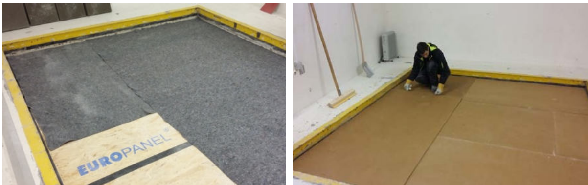
Fig. 19: Measurement of the impact sound insulation of a selected floor structure composition
