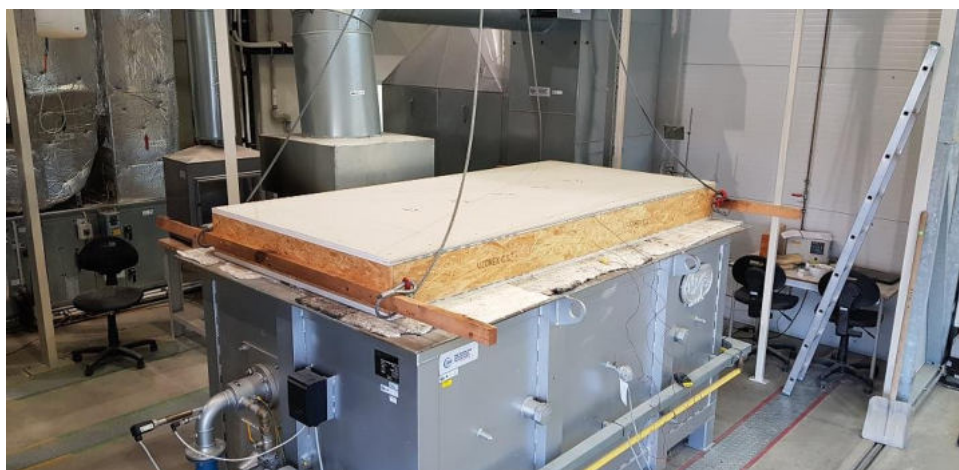
Fig. 4: Testing the fire resistance of a wall element structure of wooden construction with an integrated thermal insulating layer inside the element.
