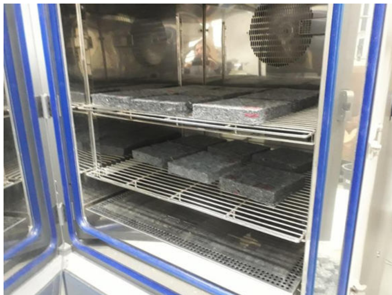
Fig. 3 Photo of samples of textile insulation with hydrophobization in a chamber providing a controlled atmosphere (development of new materials with the company Retex)
