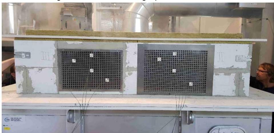
Fig. 5: Testing the fire resistance of fire ventilation grilles in which segments that expand during the increase of the temperature and prevent further spread of the flame through the ventilation grilles, are integrated.
