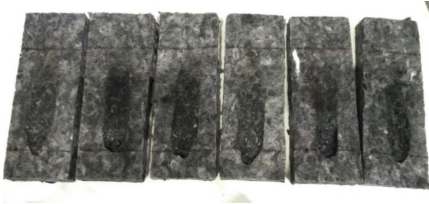
Fig. 9: Samples of heat insulating material after testing the reaction to fire - flammability of construction products exposed to direct flame - small flame source.
