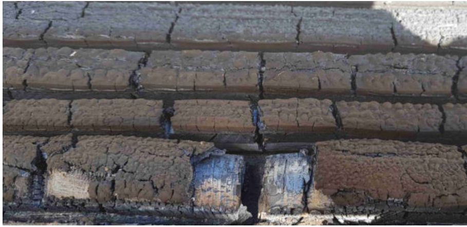
Fig. 6: View of a wooden acoustic panel sample after the test, with an expanded fire coating on the surface
