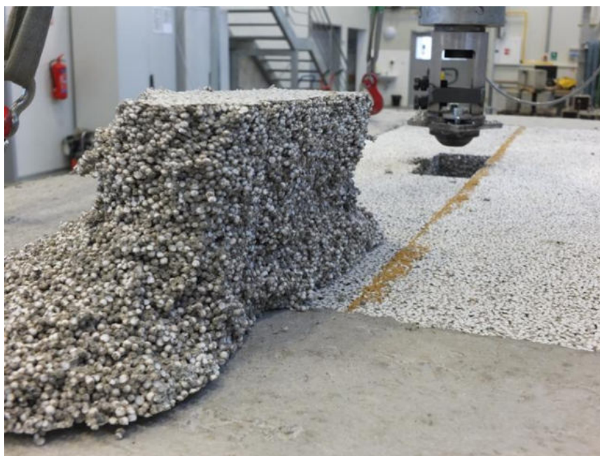
Fig. 2 Photo of a polystyrene concrete sample after the bearing strength of the filling of the reinforced concrete panel was tested (in cooperation with the company 3isolet)
