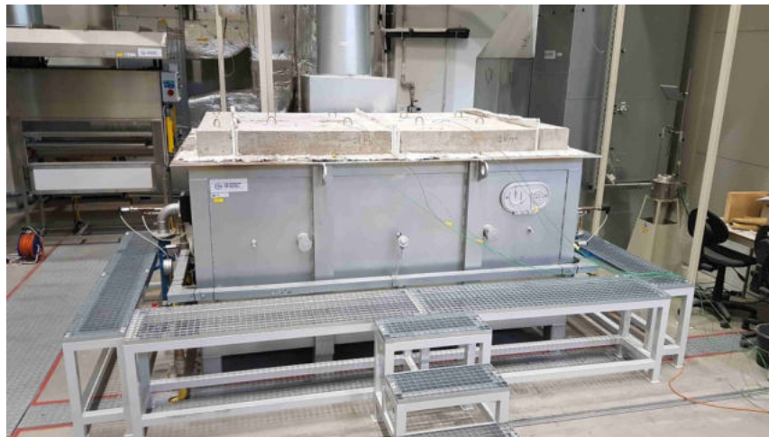
Fig. 10: Testing of the fire resistance of the thermal insulator in a reinforced concrete slab and monitoring the temperature development inside the element for 120 minutes at high temperatures (up to 1100 °C) - view of the stored sample during the test
