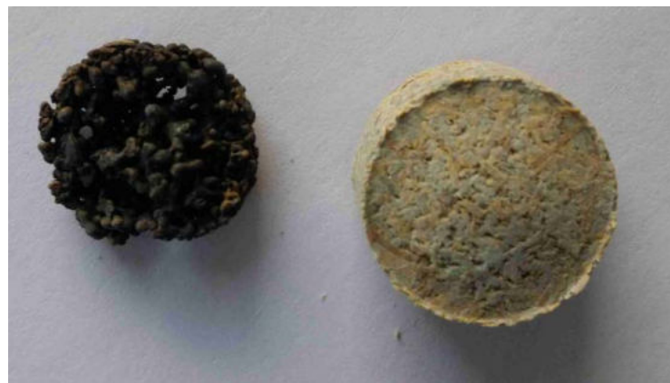
Fig. 8: A detailed view of specimens of cement-bonded chipboard after the test (left) and before the test (right) for determining the heat of combustion which is part of the fire performance classification tests.
