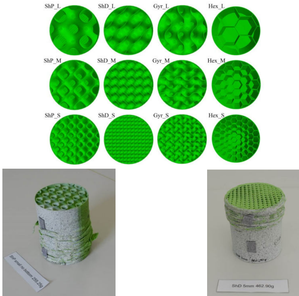
Fig. 38: Overview of the studied structures of fillers used in construction components (above) and an example of the resultant shapes of two selected samples after a compression loading test.
