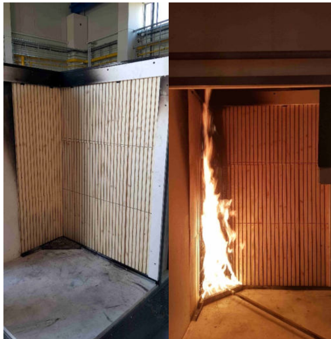
Fig. 7: Wooden acoustic panels prior to the test and during the test of determination of the reaction to fire, specifically with the action of a single burning object. Both pictures show test specimen mounted on a test rig truck that is loaded into a test chamber.
