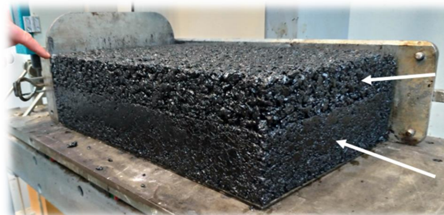
Figure 2. Lake pavement sample, with described layers (upside down)
