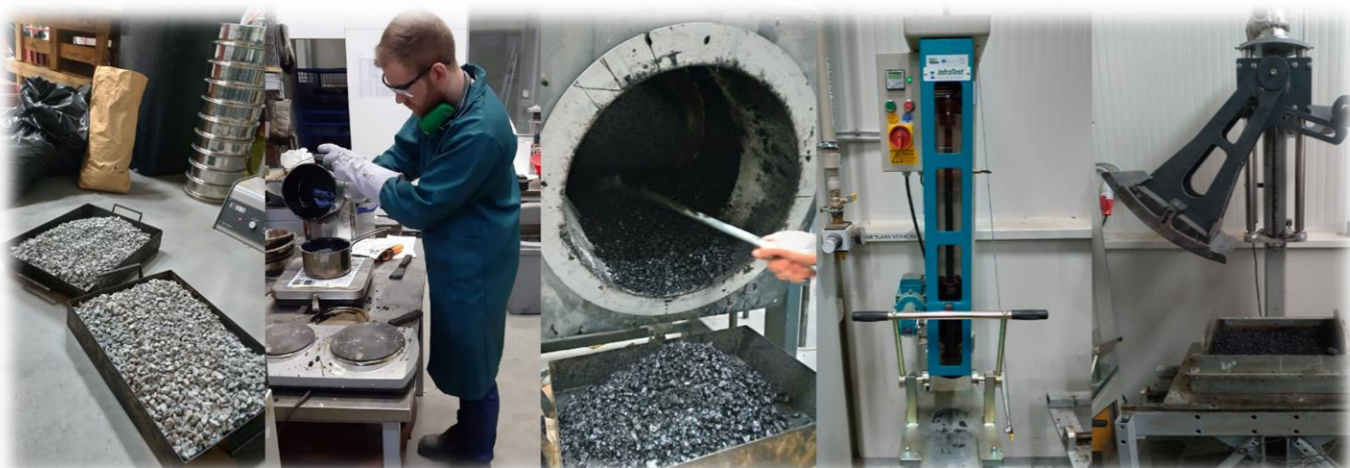
Figure 3. Preparing, mixing, and compacting the asphalt mixture
