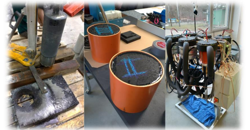
Figure 4. Drilled, prepared, and on test pavement samples
