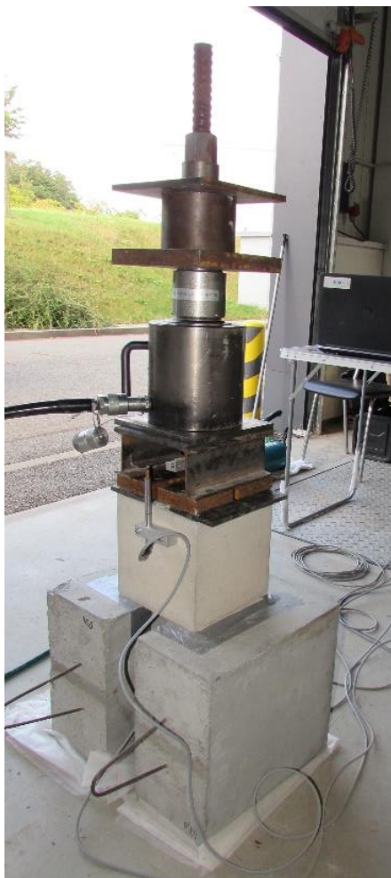
Pull-out test of the anchorage length of reinforcement (on a cube and a cylinder)
