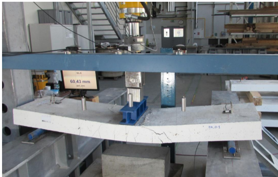
Failure of a panel with GFRP reinforcement and a span of 1.4 m
