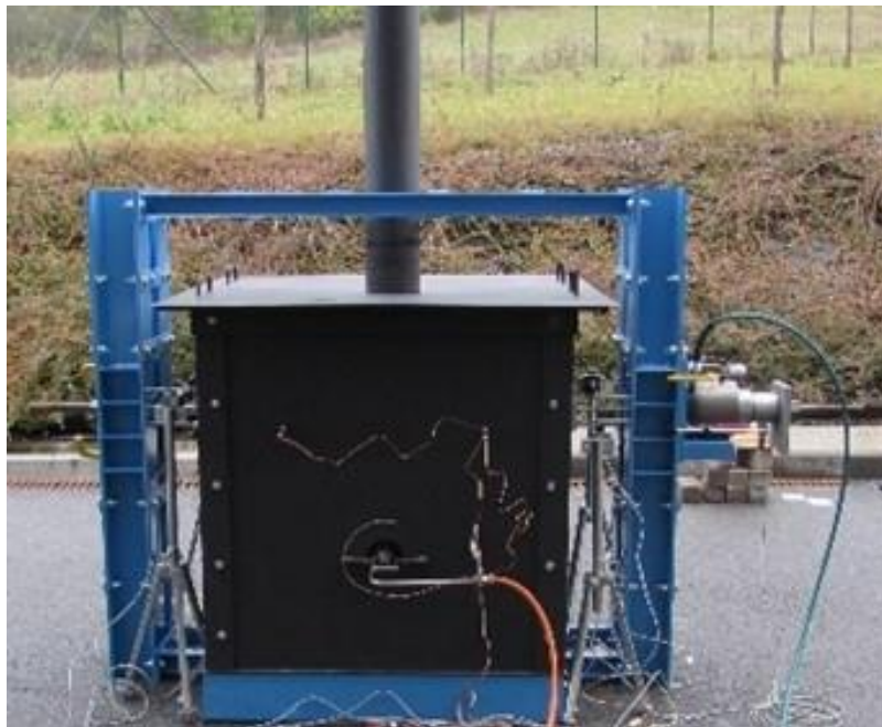
Tensile strength testing of reinforcement at elevated temperatures in a fire resistance test furnace
