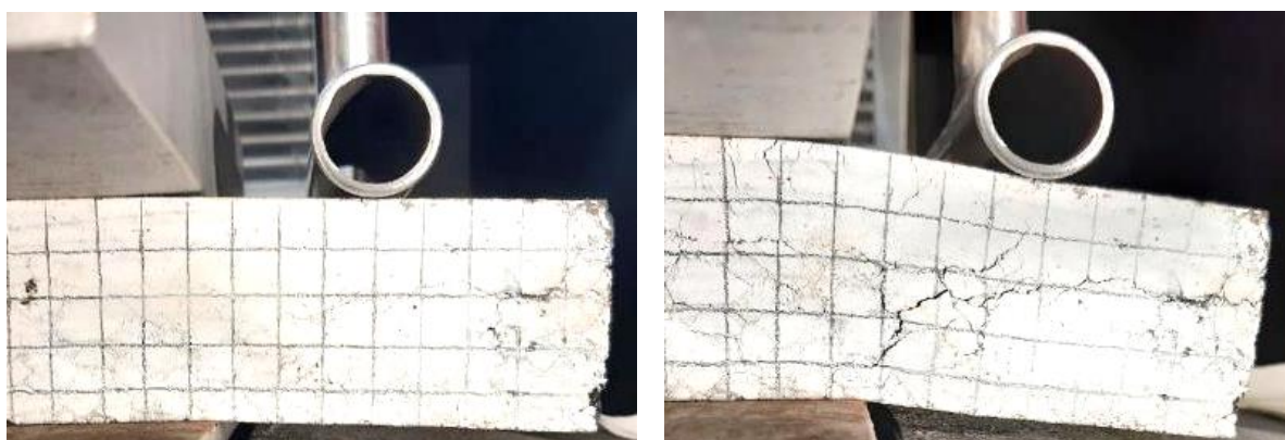
Testing of the resistance of reinforced layers against shear stress, left: at the start of the test, right: at a deflection under load of 7mm
