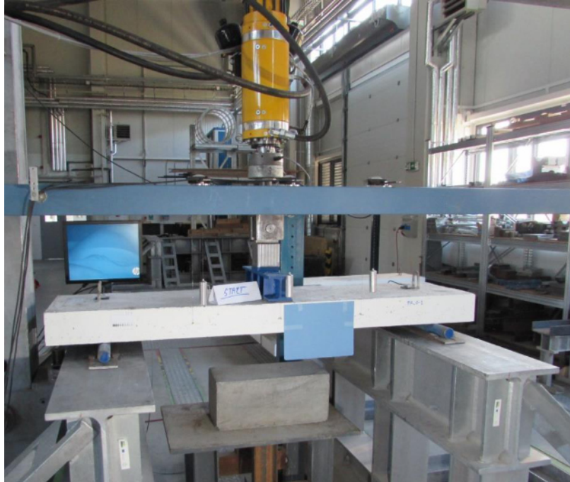
Load test of panels in three-point bending
