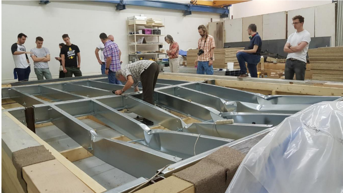
Experimental verification of one of the ceiling structure variants - illustration of the assembly arrangement and failure after ultimate strength was reached.
