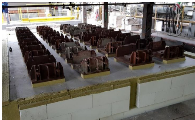
Test specimens installed in a fire resistance test furnace (figure above) and under load (figure below)
