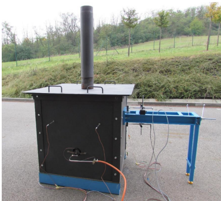
Fire resistance test furnace with a load frame for anchorage length tests
