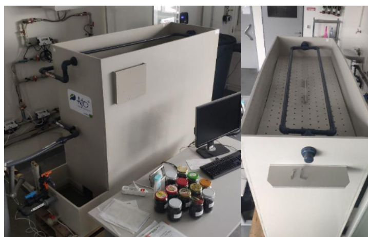
Sand filtration unit (left), and a view of the distribution plate (right)
