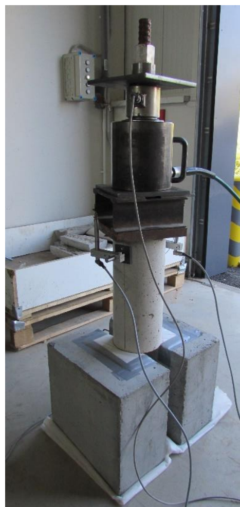
Pull-out test of the anchorage length of reinforcement (on a cube and a cylinder)
