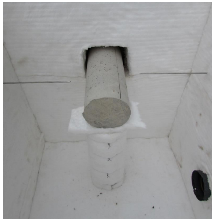
Placement of the specimen inside the combustion chamber of the fire resistance test furnace
