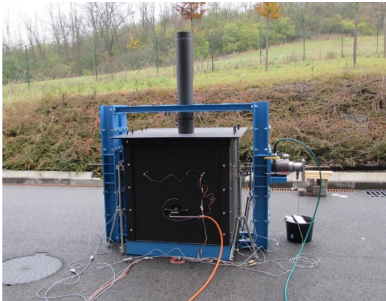
Fire resistance test furnace with a load frame for tensile tests
