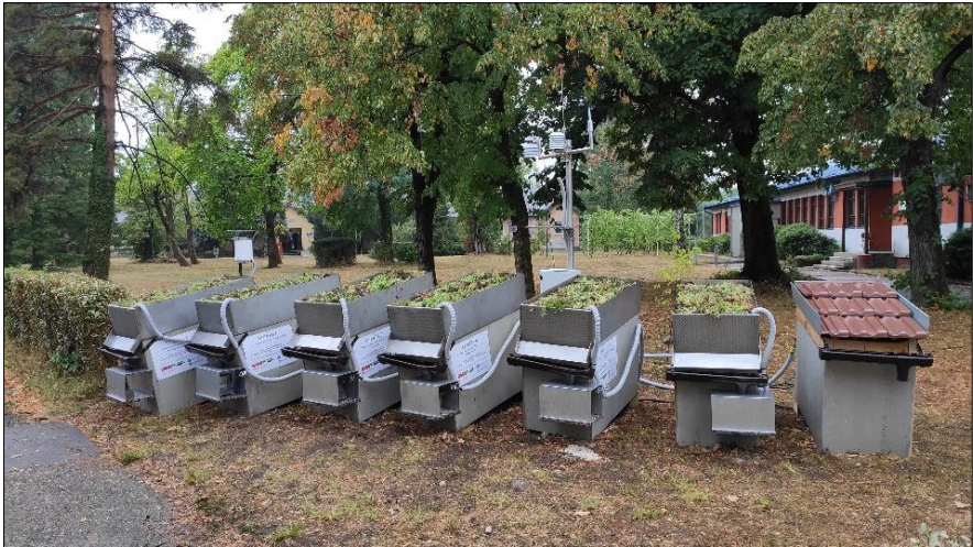
Figure 6. Experimental green roof modules in Banja Luka
