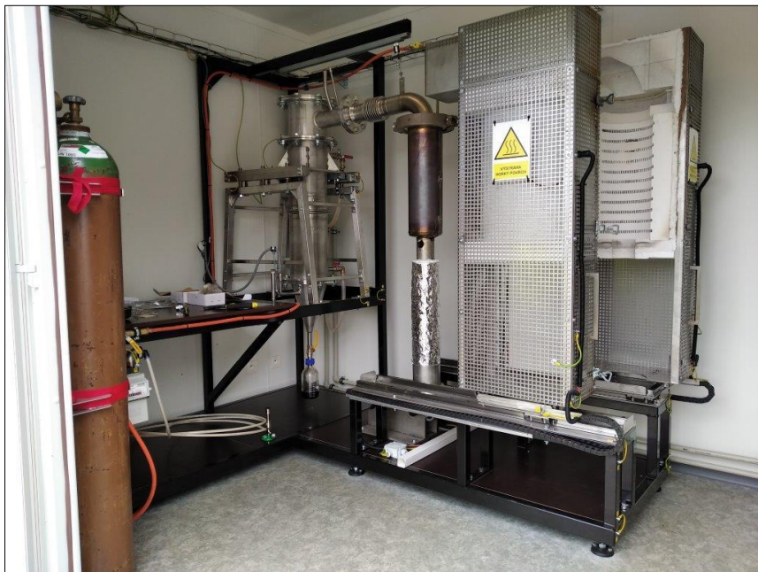
Figure 3. Thermal pyrolysis unit at AdMaS Research Centre
