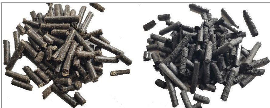
Figure 2. Pelletized (6 mm) dried sewage sludge with wooden sawdust (left), biochar from dried sewage sludge with wooden sawdust (right)
